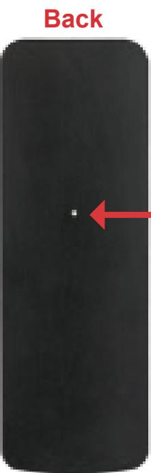
Use a pin to insert into the hole and push out the front panel PCB and remove it (be careful to avoid damaging the IR LED)
